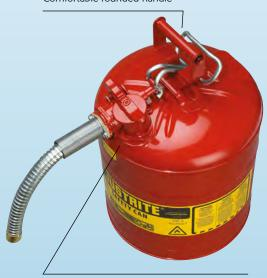
The built-in pressure relief valve automatically prevents a bursting of the container in case of heating. Self-closing flexibly mounted cover prevents leakage of vapours and inadvertent discharge of hazardous liquids.
